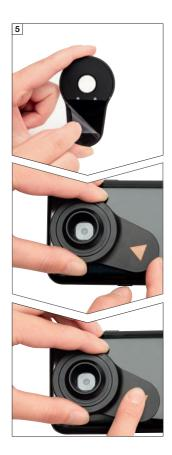
Remove the protective film and press the connector firmly over the centre of the selected camera lens.
