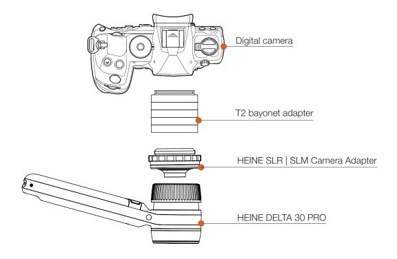
Enhance your HEINE dermatoscope with the SLR | SLM Camera Adapter. The combination of the HEINE DELTA 30 or HEINE DELTA 30 PRO, the HEINE SLR | SLM Camera Adapter and a DSLR or DSLM camera creates a comprehensive system for documenting consistently high-quality images.
